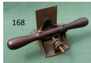
168 Stanley 12 scraper with little used 32TPI toothing iron. Comes in as found condition with dirt and surface rust. Will clean to G+ $ 70-120
