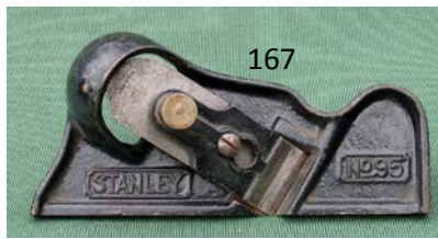
167 Stanley 95 edge trimming block plane with most of the original finish intact. G+ $ 70-150
