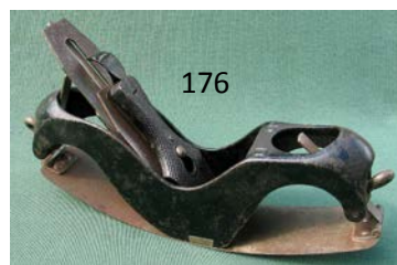
176 Stanley 13 circular plane with Pat 92 cutter. Excellent condition, minor surface rust only. G+ $ 70-140
