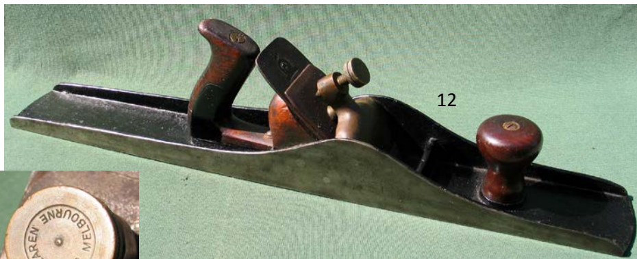
12 The star of the show: Very rare Australian plane: Jas McLaren, Melbourne cast iron 23 1/2 jointer with wooden frog. I've heard of only one other. Probably manufactured pre WW1 with a similar design used by American manufacturers as well as Spiers. Good overall but repainted, fixed handle and there is a hole in the lever cap. G $ 500-1,000
