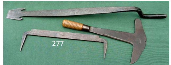
277 Great set of roofer's tools: 28" slater's ripper plus a German 13" Sombora slater's hammer and a 13" Tyzack slaters anvil. All G+ $ 80-120
