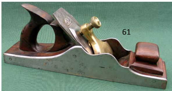
61 Buck dovetailed steel 13 1/2" panel plane with rosewood infill and closed handle. Comes with a 2 3/8" parallel iron by Hearnshaw. It's generally assumed that most of the Buck planes were made by Norris. Minor storage rust, small fix to handle spur G $ 200-400
