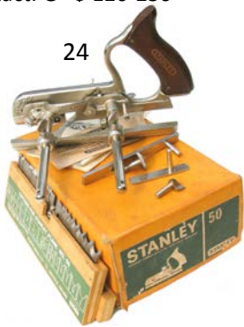
24 Stanley 50 plough plane made in England. Guaranteed complete with all attachments including chip deflector and screw for small cutters as well as a full set of cutters. F $ 80-130
