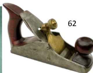
62 Curious looking smooth plane with steel sides and brass lever cap. 8 1/2" long. Fr $ 20-50
