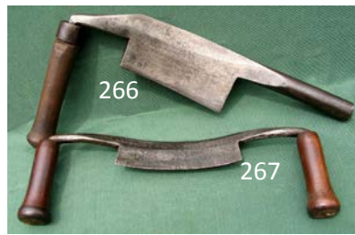
266 Large 18" cooper's jigger / chamfering knife with 6 1/2" cutting edge by Barton. G $ 40-80
