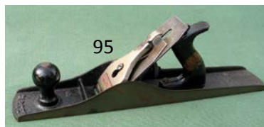
95 Carter 06 jack plane with most of the original finish intact. Small rust/pitting spots side and sole. G+ $ 30-60
