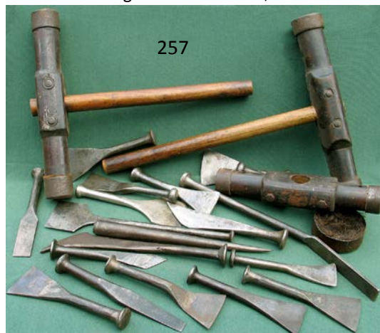
257 Great set of shipwright's tools. 3 caulking mallets, 16 caulking irons plus a marlin spike. G/G+ $ 200-400
