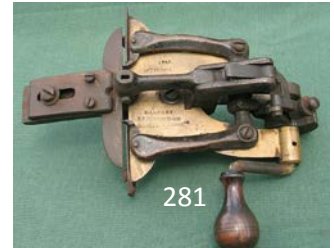
281 Early Cunningham gunmetal bodied saw shaper/swage tool patent Dec 23, 1873. G $ 70-140
