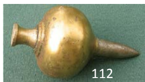
112 8oz Germanic turnip shaped brass plumb bob with steel tip. 3" long. G $20-40
