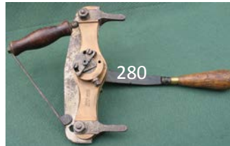
280 Brass saw shaper/swage tool marked Fleet shaper Pat 108399. 9" long G $ 50-100
