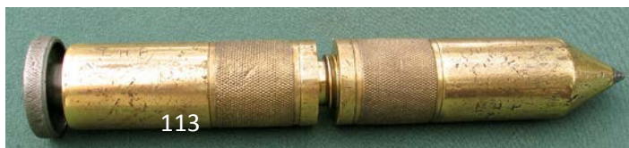
113 Unusual brass double plumb bob. Top part unscrews to make it a 1.25kg or a 2.25 kg. Shown slightly open, the two parts screw together tightly. 10" long. G $ 30-70
