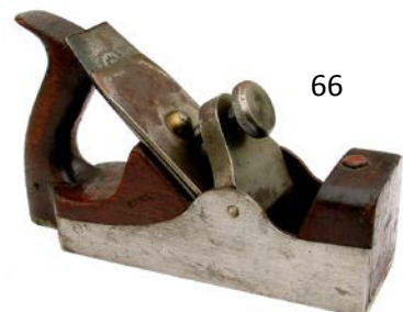
66 Custom made cast iron infill smoother with 2 1/4" Mathieson cutter. 9" long. G $ 30-60
