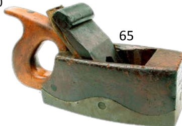
65 Early transitional smooth plane with cast iron base, beech infill and wedge and closed handle. 9" long G $ 30-60
