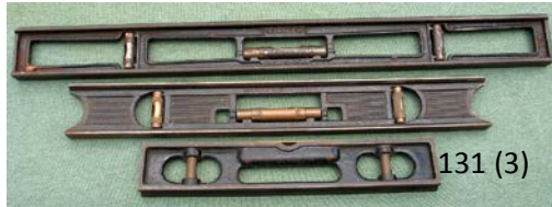
131 Two Stanley and one Rabone level 24", 18", 12". First one with small fix, all of them have one vial dry or broken. G- $ 30-50
