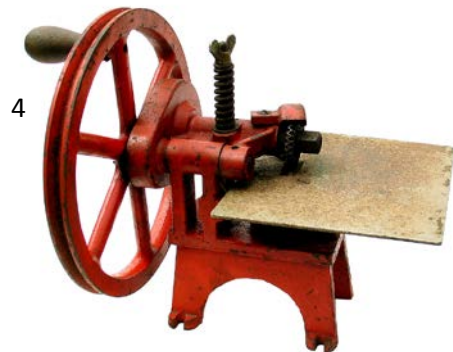
4 Cast iron edge cutting machine or crimper. Cuts a serrated edge – I guess for tin or similar. VG working order. 13" x 11" x 12" G 50-100
