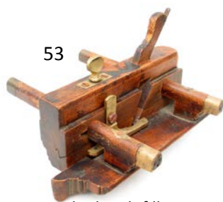
53 Unmarked sash filletster. No nicker, no stem – or nicker wedges. G- $ 30-60
