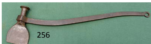
256 Very rare shipwright's hawsing axe i.e. a handled caulking tool. 27" long with a 4" working edge. G $ 70-140
