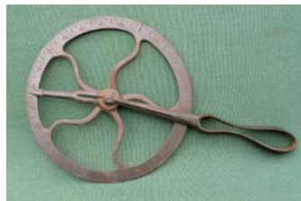
135 Very good factory made blacksmith or wheelwright's traveller with indicator. No maker's mark. G $30-60
