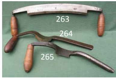
263 Curved cooper's drawknife by Gilpin. 12" cutting edge. G $ 30-50
