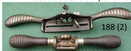
188 A Stanley 66 beader with router bit and fence and a Stanley 67 universal spokeshave with round sole. G $ 30-60
