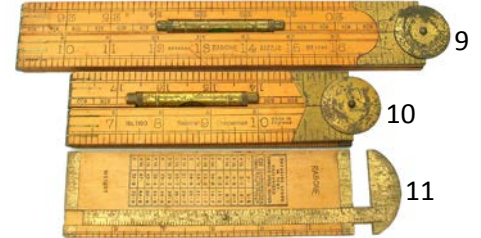
9 Rabone 1190 four-fold 3 feet boxwood combination rule with level and clino. G+ $ 25-50
