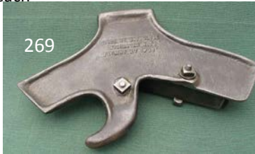
269 Cast iron 13" cooper's chiv by C.F. Close, Rochester N.Y. Pat 1913. Unusual tool. G $ 50-100
