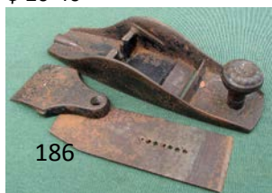
186 Leonard Bailey Victor block plane parts. Body knob and blade good, lever cap comes with wrong screw. Fr $ 40-60
