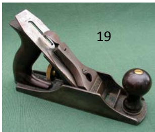
19 Bedrock 603 smooth plane with one line Bedrock lever cap and SW cutter. Some rust, very minor pitting marks and loss of japanning G $ 100-200
