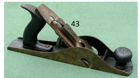
43 Stanley 10 made in USA with good rosewood handle and low knob. T logo cutter has been repaired. Dark spots are dried grease. Should clean to G $ 50-100
