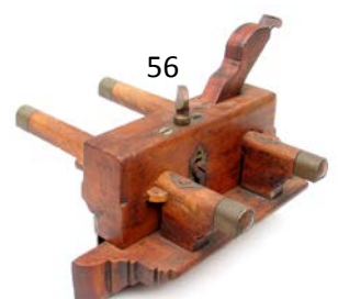
56 Plough plane by Atkin & Sons. One stem wedge damaged. G- $ 20-40
