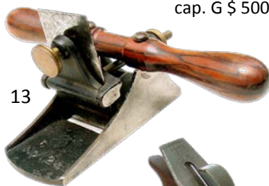
12 The star of the show: Very rare Australian plane: Jas McLaren, Melbourne cast iron 23 1/2 jointer with wooden frog. I've heard of only one other. Probably manufactured pre WW1 with a similar design used by American manufacturers as well as Spiers. Good overall but repainted, fixed handle and there is a hole in the lever cap. G $ 500-1,000
