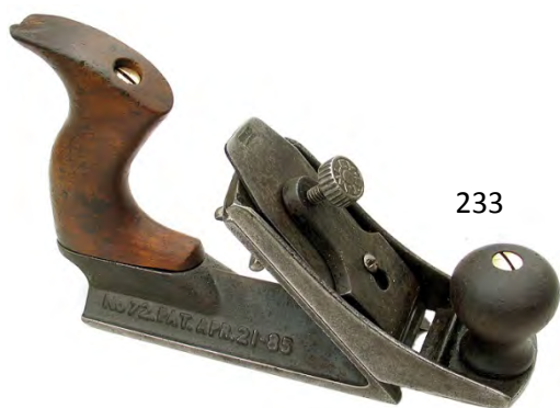
233 Stanley 72 chamfer plane with pat 95 on side. Tight hairline crack in handle. Cutter is Stanley and looks correct but it's from a block plane. Not much japanning left. G- $ 100-200
