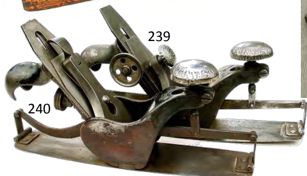
239 Early Stanley 113 circular plane with side wheel adjuster. Pat 92 cutter. Some paint marks on sole, overall G+ $ 80-150
