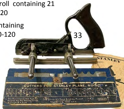
31 Stanley 50S made in England. Economy model with reduced set of 8 plough cutters, chip breaker and holding screw for small cutters. Plane G+, box G- $ 50-100
