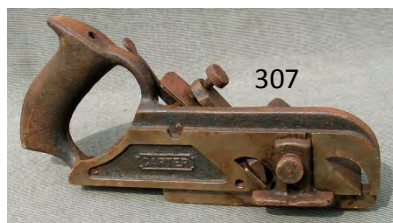
307 Carter 78 rebate (duplex) plane with fence and depth stop. G $ 20-50
