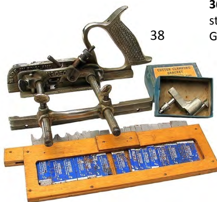
38 Record 050 small combination plane with 17 cutters, chip breaker and small blade holder, depth stop and beading stop. G+ $ 50-100
