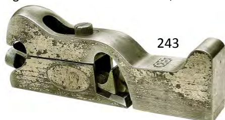
243 Stanley 93 rebate plane made in USA. Two patents to 1900 on cutter. Loss of plating and hairline crack where the top screw bolts the two parts together. P $ 30-60
