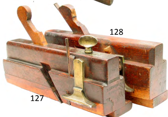
127 Moving filletster with dovetailed boxwood sole by I. Lund, London 1805-1831. Nicker wedge replaced. G $ 30-60
