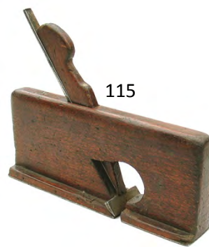
115 7" T-rabbit with steel sole. Scratch one side and splinter off the wood sole (the steel sole might actually be a fix) G 10-20
