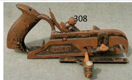
308 Stanley 78 rebate (duplex) plane with fence and depth stop. Fence screw is a replacement. G $ 20-50
