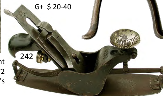
242 Ohio Tool Co compass plane. Same as Stanley 113 but comes with a superior, much thicker tapered Ohio cutter. G+ $ 80-150
