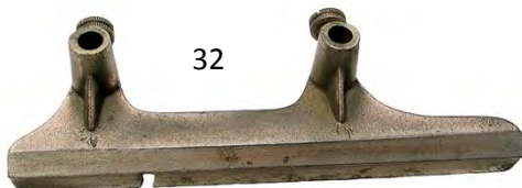
32 Fence 6H for Stanley 45 combination plane. Round slotted screws. G $ 20-40
