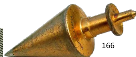
166 Scarce surveyor's brass plumb bob by Stanley London. Long neck and screw with domed finial. 4 1/2 " long. Still has original finish. F $ 30-60
