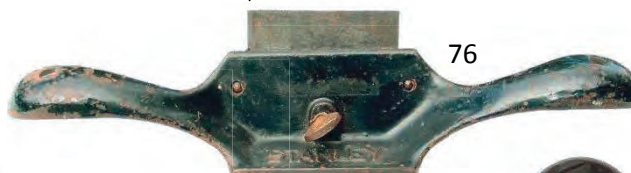
76 Stanley 80 cabinet scraper made in USA. SW logo on strap and on cutter. G 20-40
