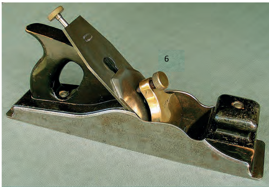
6 Norris 14 1/2" panel plane. Post war model with beech infill and handle. Excellent plane in as found condition with a full Norris cutter, clean sides and sole and only minor wear to the black finish. G+ $ 900-1,400
