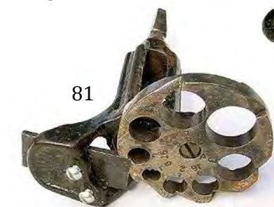
81 Adjustable Hollow Auger with selector wheel by Stearns. About 3/4" of the original finish is intact. Complete with depth stop. The screws that hold the cutter are fitting replacements. G $ 30-70
