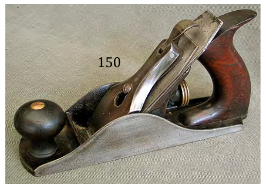
150 Pre-lateral Stanley 3 smooth plane type 2 with solid brass adjuster nut with the early Bailey patents. Pat 1867 cutter and correct pat 67 back iron; correct flat-back lever cap; beaded front knob and early rosewood handle. There is one neat owner's mark on the neck of the lever cap as well as along the base of the l/h side. Approximately 90% japanning is intact. Some Minor rust spots one side and sole. G+ 100-200
