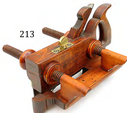
213 H. Browning, Rowe Mass 1850-55 beech plough plane with boxwood stems. Virtually no stem damage. G $ 60-120
