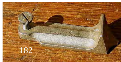
182 Blade clamp/chip breaker for Stanley 90 bullnose or Stanley 93 rebate plane, free of chips or cracks. G+ $ 20-40
