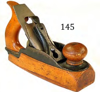
145 Pre-lateral Stanley 35 transitional smooth plane with eagle trademark on toe. Correct J logo cutter. No chips or cracks, a very collectable tool with good patina and most of the original finish intact. G+ 60-130
