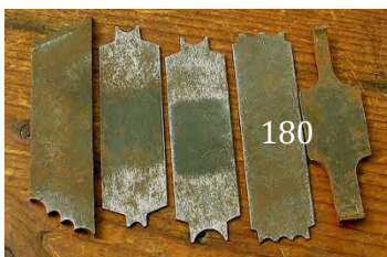
180 Lot of five cutters for Stanley 66 beader. 4 are Stanley, one is custom made. The router cutter is marked Stanley. G $ 25-50
