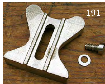
191 Fence with screw for Stanley 71 router. G+ $ 15-30
