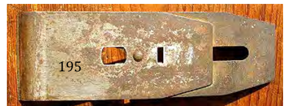
195 very little used Stanley 8 cutter and back iron with Pat 92 logo. Surface rust only, this one will clean to G+ $ 25-40
