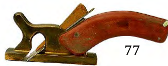
77 Small coachmaker's brass T-rabbit plane with squirrel-tail epoxy handle. Few small chips on mouth. Could look stunning with a better wedge & wood handle. Plane is 3 1/4" long without handle. G $ 40-80
