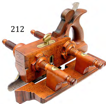
212 Mathieson 9B beech plough plane with closed handle and boxwood stems and nuts. One of the inner nuts is cracked (fixed) otherwise G+ $ 100-200
