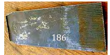
186 2" Tothing cutter with good length serrated edge for veneering work. Maker is Buck Bros. G 10-20
