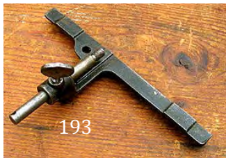
193 Fence with rod and correct thumb screw for Stanley 78 rebate plane. G $ 15-30
