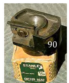
90 5/16" cutter head for Stanley 77 rod and dowel turning machine. G+ $ 50-90
