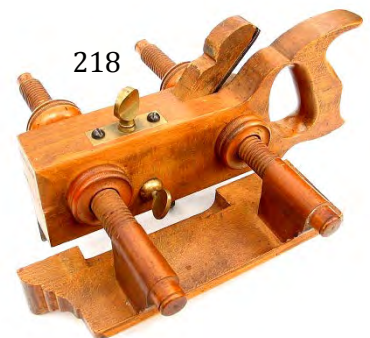
218 AC Bartlett's Ohio Planes mark on this beech plough plane No 119. Manufactured by the Sandusky Tool Co for Hibbard, Spencer, Bartlett & Co 1890-1920. G $ 60-120
