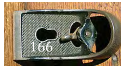
166 Stanley block plane lever cap to fit most adjustable models incl. 9 1/2, 220 etc. Some loss of japanning. G $ 10-20
