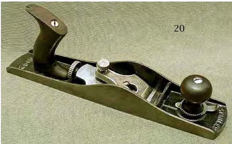
20 Stanley 62 low angle plane. Perfect sole and mouth, some minor loss of japanning to the rear of the handle (paint touch-up), hairline crack in handle. G+ $ 220-450
