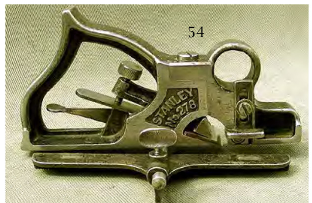
54 Stanley 278 rabbit & filletster plane with correct fence and depth stop. Depth stop screw is not original. Pat 12-17-16 on cutter, approximately 80% japanning intact. Tiny chip on outer rim of the fence rod receiver. G+ 150-300
