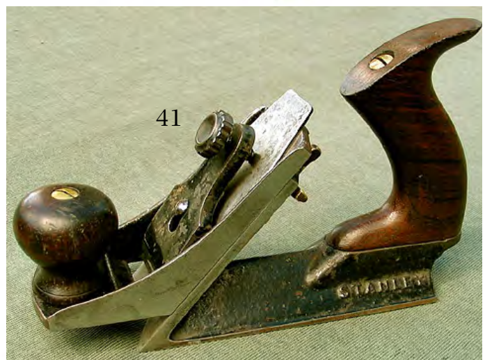
41 Stanley 72 chamfer plane, marked Stanley on one side and # 72 on the other with the early lever cap screw, indicating this plane was made between 1885-1905. Cutter is a matching replacement from an early Stanley Excelsior block plane. VG rosewood, correct beaded front knob, approximately 80% japanning intact. G+ $ 200-400
