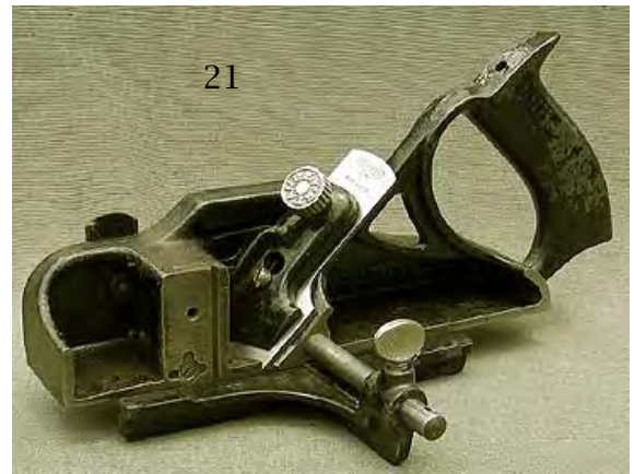
21 Stanley 289 skewed filletster and rebate plane, all parts present and correct. SW cutter. Approximately 70% japanning intact, no rust or pitting. G+ $ 150-300
