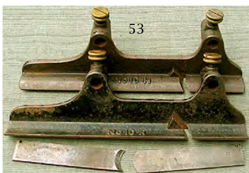
53 Pair of #10 Hollow and Round fences for Stanley 45 combination plane with slotted brass screws and new cutters. One lost most of the japanning. G $ 50-100
