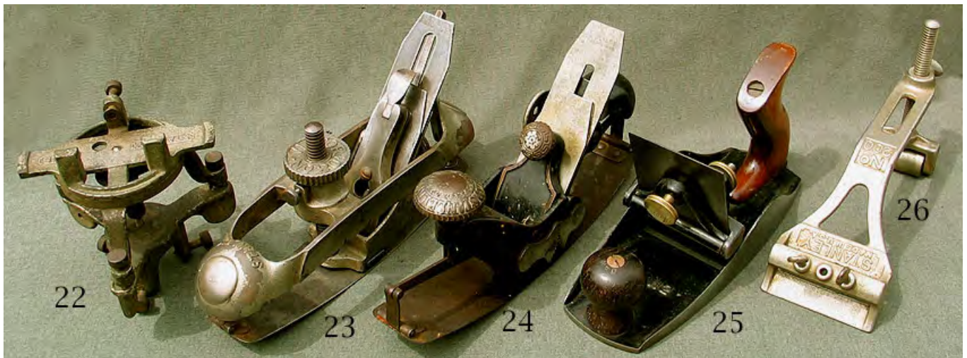
22 Stanley 48 level stand, takes levels up to 1 3/8" wide. Complete with correct screws, nickel plating dirty but will clean to G+ $ 60-120
