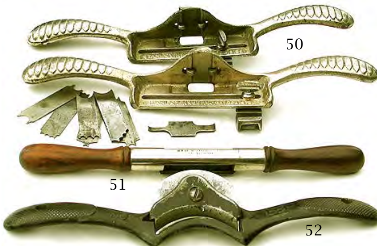
50 Pair of Stanley 66 hand beaders, both with patent 1886 on front rail, one with round fence, one with straight fence. Total of 8 cutters included, most of them original Stanley. G/G+ $ 60-120
