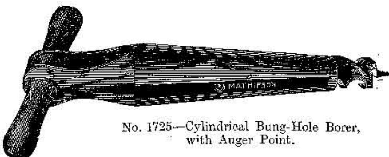
No. 1725—Cylindrical Bung-Hole Borer, with Auger Point.
