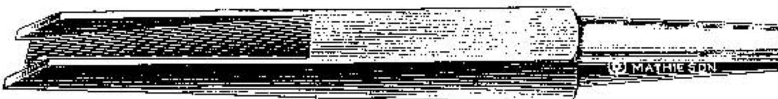
Grooved Back or Self-Coring Mortising Chisel.
