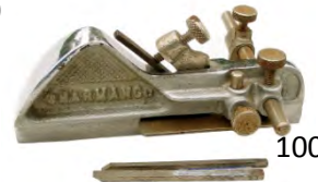
100 Sharmanco, small Australian plough plane with depth stop, fence and 3 cutters ( Record) G $ 15-30
