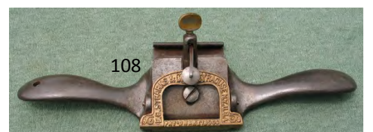
106 Early Stanley 62 reversible spokeshave. Both cutters with early R&L logo, pat applied inside handle. G $ 40-80
