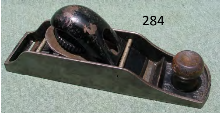
284 Stanley 130 double ended block plane made in England. G $ 20-40
