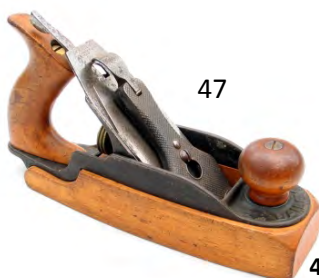
47 Stanley 35 transitional smoother. V logo cutter low. Most japanning intact. Nice, clean wood. Lever cap slightly narrowed down on both sides. G+ $ 40-80
