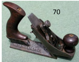
70 Stanley 72 chamfer plane. Pat 95 on side. R&L cutter, approximately half japanning. Good rosewood handle, knob has minor crack to base. G $ 120-240
