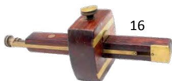
16 Rosewood and brass mortise gauge No 98 by Disston. Pins low. G $ 20-40
