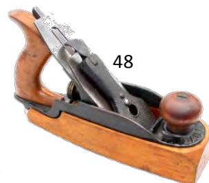
48 Stanley 35 transitional smoother. T logo cutter, hardwood mouth insert. Clean plane G $ 40-80
