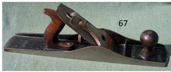
67 Stanley 6 made in USA fore plane. 90%+ japanning, good rosewood. Lat model lever cap, SW Can cutter. G+ $ 50-90
