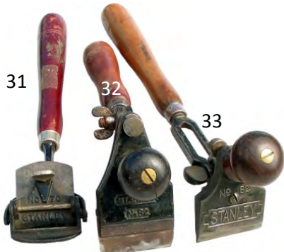
31 Stanley 70 box scraper, later model with red handle and model number on the cap. G+ $ 25-50
