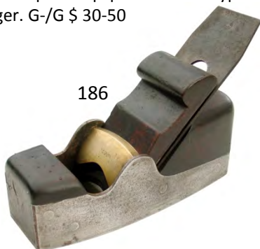
186 Early Spiers 7 1/2" dovetailed steel coffin shaped smoothing plane with rosewood infill and rosewood wedge behind brass bar marked Spiers Ayre. These early wedge type infill planes are rare. G+ $ 200-400
