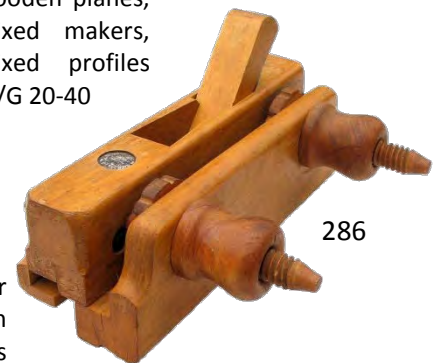
286 Screw-stem plough plane with Yugoslav maker's mark. Full length wooden depth stop and fence. G+ $ 40-80
