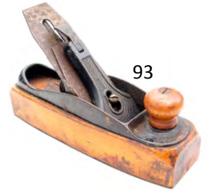
93 Sargent 3409 smooth plane with added brass sole. Discolouration and dirt. G $ 20-40
