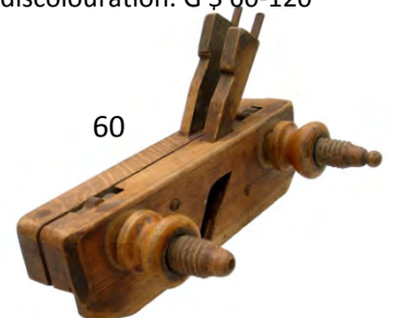
60 Custom modified (compassed) double sided screw stem sash plane by Ottokar Skrivan, Prague. G $ 50-100
