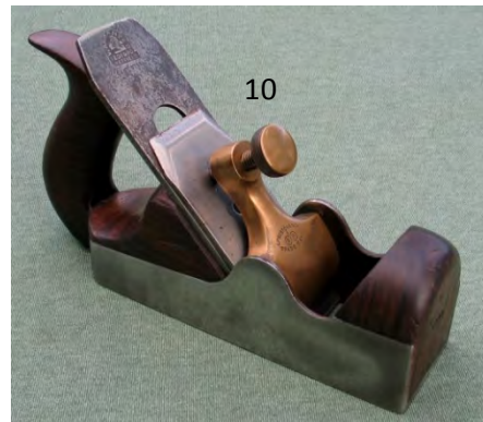
12 Mathieson ¾" dovetailed steel rebate plane with rosewood infill and wedge. Sneaked cutter by Howarth. Minor rust marks. G $ 100-200
