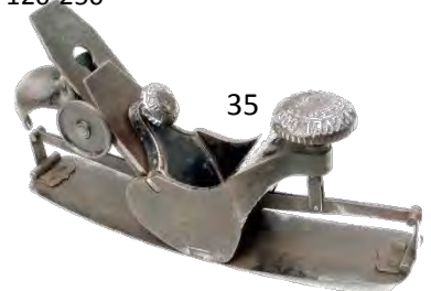
35 Stanley 113 circular plane, early model with solid side wheel. Japanning inside good, outside all but gone. Type 1 cutter. G $ 70-150
