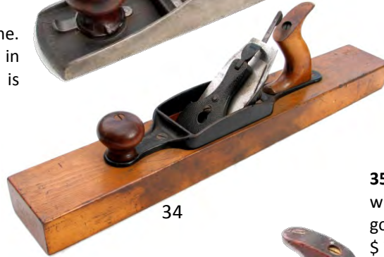
34 Stanley 30 jointer plane (22" long). Cutter low, some scratches on sole and some discolouration to one side. Overall still G+ $ 60-120
