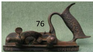
76 Early Stanley 50 small plough plane with patent 83 on fence. One cutter, no depth stop. G $ 20-40
