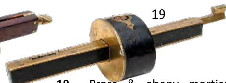
19 Brass & ebony mortise gauge. 8" long with brass top and bottom on slide. Lacquered. G+ $ 40-80
