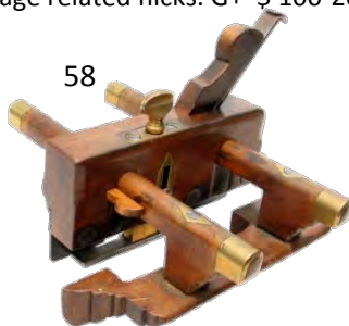
58 Small coachmaker's plough by Holland. Replaced stem wedges. G+ $ 20-50
