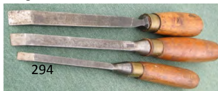
294 3 English mortise chisels 1/4", 3/8" & 1/2". Two handles ill fitting. G $ 25-50
