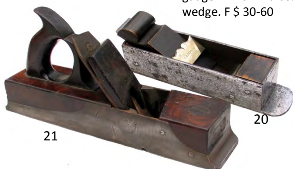
20 Custom made steel mitre plane, wooden core with steel face plates and sole, secured with screws. Nice brass cross-bar. Steel has pitting marks, sole and mouth are acceptable, cutter is basic. Could be improved. Fr $ 50-100
