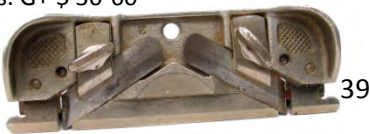
39 Stanley 79 made in UK side rebate plane with fence. Comes in custom made wooden box. F $ 40-80
