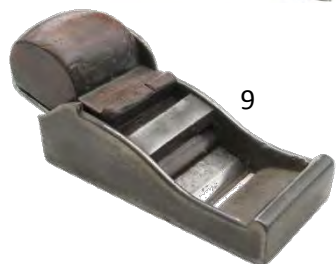
9 Cast iron chariot plane 5" x 2" with mahogany wedge behind steel bar. Top of the r/h casting broken off. Fr $ 30-60
