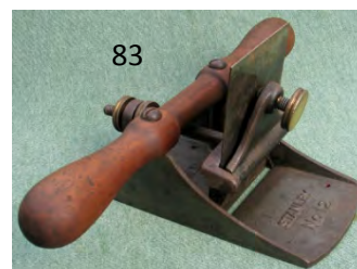
83 Stanley 12 with two (fence) holes drilled in sole. Bed stripped, maple handle. Non-Stanley cutter. Fr $ 30-60
