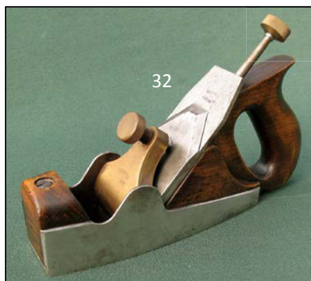
32 Norris A5 post-war smoothing plane with low Norris cutter. Lateral adjuster probably is a replacement. Good user plane, just re-bit the cutter. G $ 250-450
