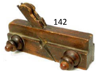
142 American window sash plane with boxwood stems and nuts. Bruising to wedges and a few cracks to side and sole. G- $ 30-60
