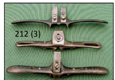
212 Three Preston shaves, ovolo, chamfer and rebate, all with Preston cutters. G $ 50-100
