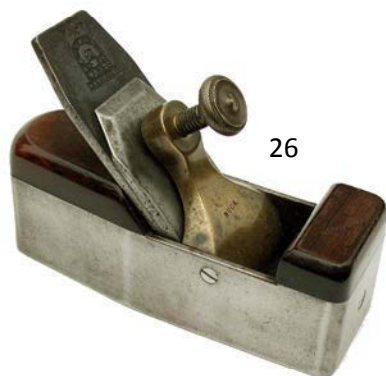
26 Buck malleable iron coffin smoother, 6 3/4 " x 2 3/8" with rosewood infill and a very good Ward parallel cutter. Little used tool. G+/F 250-450
