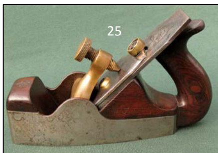
25 Spiers dovetailed steel smoothing plane with rosewood infill and handle. Well disguised hairline crack in handle and filled spot on front bun from old strike button. Mathieson cutter with custom added lateral adjustment knob to back iron. G $ 200-300
