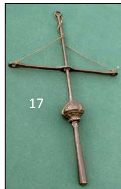
17 16" stonemason's iron pump drill with simple chuck for square shanked drill bits. Probably 18 th century. G 50-100
