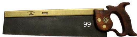
99 Mathieson 14" brass-back tenon saw with very good markings on back and handle. Minor rust spots. G+ $ 30-50
