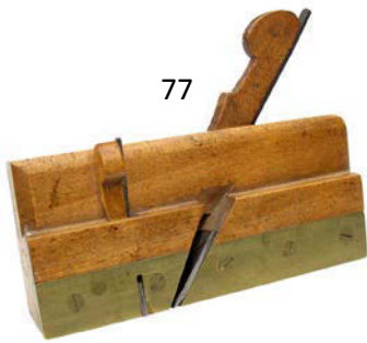
77 Rare Mathieson shouldering plane with brass side and nicker with boxwood wedge. 7" long. Little used. Listed as No 841 in early Mathieson catalogues. (often sold as dovetail planes) F $ 50-90
