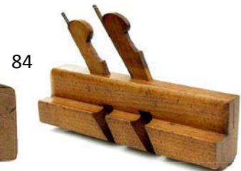
84 Early Mathieson double iron moulder with custom altered (sash) profile. G $ 60-120
