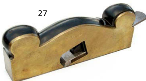
27 Gunmetal shoulder plane, 8" x 1 3/8" with steel sole. Ward cutter. No maker's mark. G+ $ 120-250
