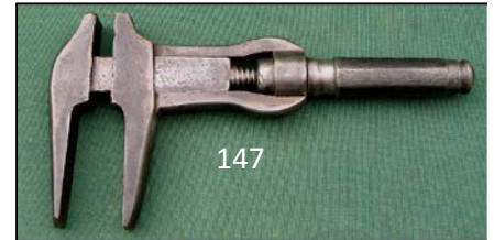
147 Most unusual 12" wrench with 3 1/2 " calliper jaws. Trademark pictured below, some more markings on top. G $ 30-60
