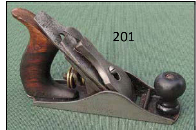
201 Stanley 1 smooth plane. Enlarged mouth, wrong front knob, some pitting on cutter, otherwise not a bad plane at all. Fr $ 200-400
