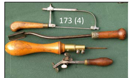
173 Jeweller's piercing saw, a long (hoof) paring tool, a Mathieson keyhole saw and a Stillman's patent 1848 saw set, all G+ $ 30-50
