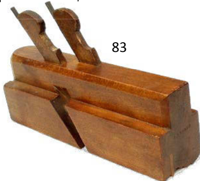
83 Complex Mathieson astragal with reverse ogee. Marked No 174 5/8 on heel. Plane is 2 1/4" wide. G+ $ 50-100
