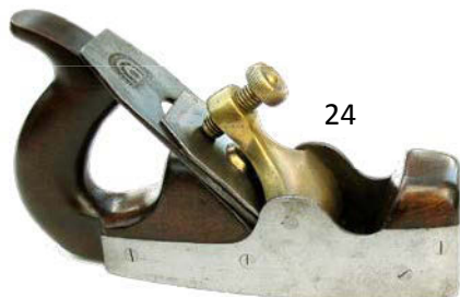
24 Spiers steel smoother with mahogany infill and open handle. Fitted with a tapered Mathieson iron. 7" base. Clean plane. G+ $ 200 - 300
