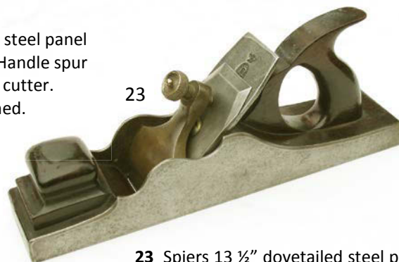
23 Spiers 13 1/2" dovetailed steel panel plane with rosewood infill and closed rosewood handle. Outstanding wood on this plane. Steel sides have some mild rust/pitting spots, a bit more on the sole but all less than 1 mm deep. Fitted with a worn Ward parallel iron. A little effort will make this plane F $ 400 -800
