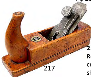
217 European horn plane marked LW with adjustable mouth and 45mm double iron by Berg with Shark brand logo. Cutter has 1/2" left under the slot. Some scratches on sole. G- $ 20-40
