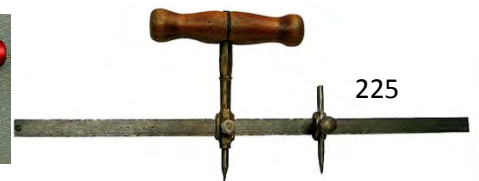
225 Large circle cutter with 19" bar, brass point with wooden handle and quality splitter. Marked Bost, France. G $ 30-60
