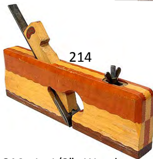
214 1 1/8" Wooden rebate plane with laminated body and adjustable mouth by Danish maker Bendixen JPBO with Berg Shark brand cutter. F $ 25-50
