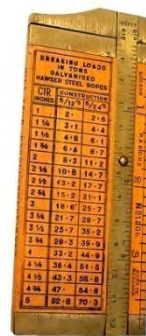
59 Rabone 1206 boxwood rope gauge with brass slide. Dutch company name on side. F $ 25-50
