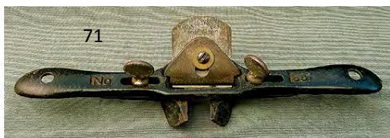
71 Stanley 65 chamfer shave with R&L cutter. Most japanning is intact. G+ $ 50-100
