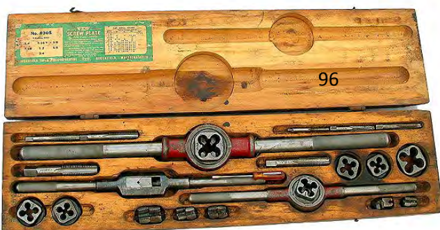
96 Large Greenfield No 8305 screw plate tap and die set sizes 1/4, 5/16, 3/8 7/16, 1/2, 5/8 3/4 in original box 26" x 6 1/2". Little used. G+ $ 50-100
