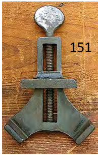
151 Preston corner clamp with 3" capacity. Maker's mark on adjuster screw. G $ 10-20
