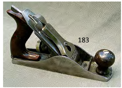
183 Stanley 3 low knob 3 patents to 1910 in bed, T-logo cutter, later SW keyhole lever cap. Very good rosewood, most japanning intact. G $ 50-90
