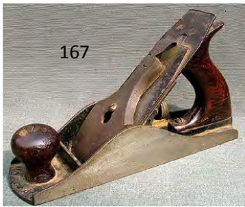
167 Stanley 4 1/2C low knob, early pre 1900 model with P trademark cutter. Most of the japanning is intact. Handle cracked with a chunk of wood missing from the spur. Some dust and dirt but overall G+ $ 60-120
