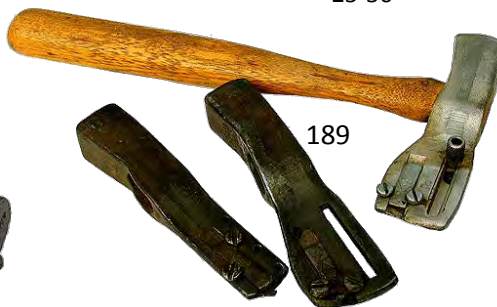
189 Lot of 3 roofing hatchets from different periods by the same US maker AJC (Anthony Joseph Crookston), all three have the patented slitter, used to cut insulation sheets on roofs. G-to G+ $ 50-100
