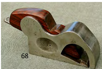
68 Preston bullnose plane with 1 1/2" Preston cutter, used down to 7/16". Very good rosewood wedge, clean mouth and maker's mark on heel. G+ $50-100
