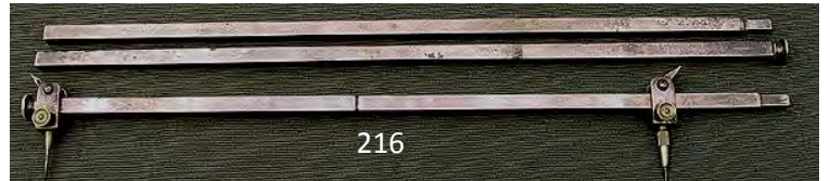
216 Long surveyor's trammel set marked David K. James. Nickel plated. 1080 mm fully extended. G $ 20-40
