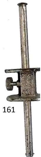
161 Stanley 97 marking gauge with pin one side and roller on the other. G $ 15-30
