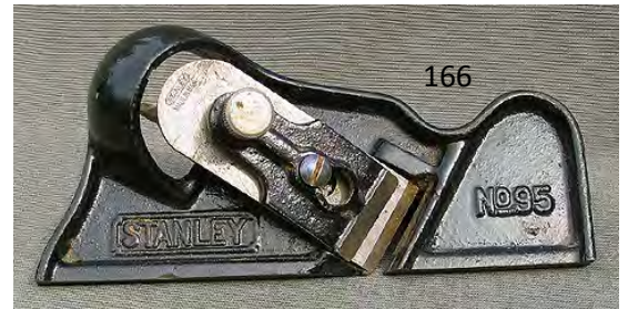
166 Stanley 95 edge trimming block plane with notched logo cutter. Tiny nick along front edge, G+ $ 70-140
