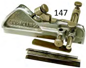
147 Sharmanco made in Australia - small plough plane with 3 cutters, depth stop and fence. G 20-40
