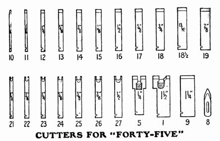
The following twenty-two cutters are furnished with each Plane. The  $\frac{1}{8}$ -inch Beading Tool and the Slitting Tool are assembled in the Main Stock: the other cutters are packed separately. The price is given in case duplicates should be required.
