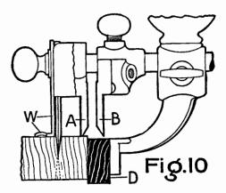
Fig. 10—SLITTING—Insert the Slitting Cutter in the slot on the right side of the Main Stock, and just in front of the Handle. Place Depth Gauge (W) over the Blade and fasten both by means of the thumb screw provided. Fence (D) gauges the distance of the cut from the edge of the board. For thick boards slit both sides.
