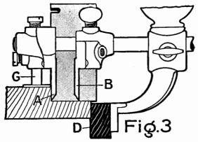
Fig. 3—RABBET AND FILLETSTER—Attach Fence (D), putting Arms through upper holes. The Fence regulates the width of the cut and if required, slides under the cutter The Sliding Section (B) also slides under the cutter, forming a support on the outer edge of the rabbet. Gauge (G) regulates the depth of the cut.
