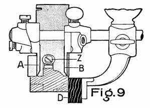
Fig. 9—SASH PLANE—The Sash Cutter is similar to the tool used for cutting the tongue on matched boards, as it has a Stop (Z) which can be adjusted to regulate the depth of the cut. One side of the moulding is cut first, the work is then reversed and the operation repeated on the other side. Fence (D) is used as in Matching. Spurs not used.
