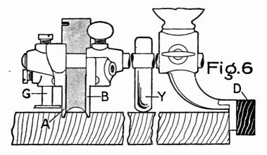
Fig. 6—CENTER BEADING—Attach Cam Rest (Y) to either Arm between Sliding Section and Fence to steady Plane. Attach Fence as in Fig 4, and Plane will cut bead five inches from edge of stock. Set as in Fig. 6 and it will cut bead eight inches from edge. Gauge (G) is used as in ordinary beading. No Spurs required.
