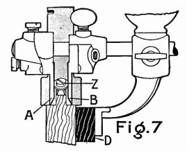
Fig. 7—MATCHING (Tongue)—Insert the tonguing cutter and set the Stop (Z) attached to same, at the proper point to obtain the height of the tongue desired. Fence (D) regulates the position of the tongue on the edge of the board. The Gauge (G) and the Spurs are not used. Boards varying from three-quarters of an inch to one inch in thickness can be matched in the center.
